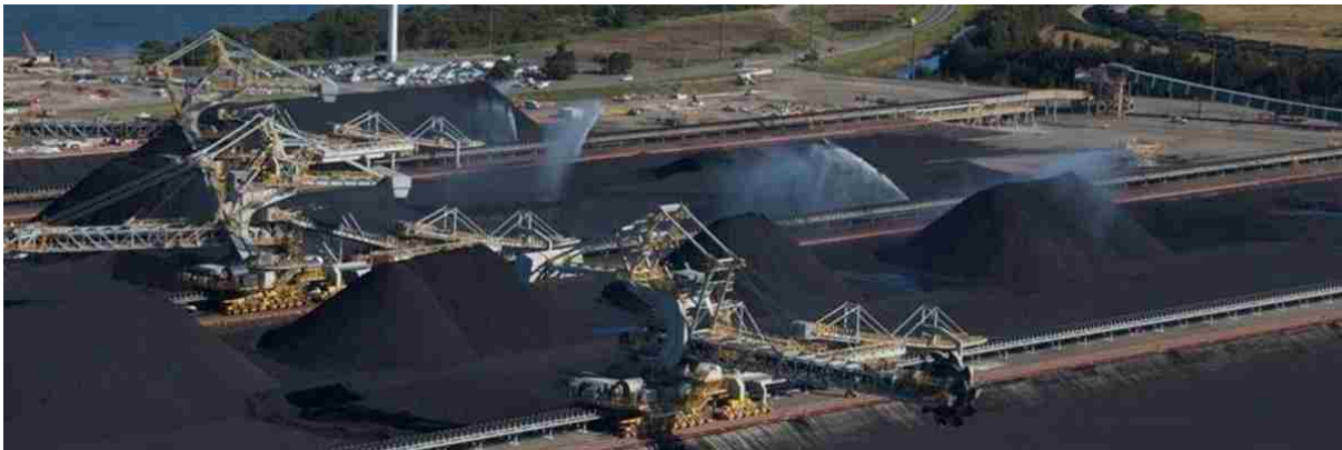
Figure 1: Watering of coal stockpiles to reduce airborne dust.
